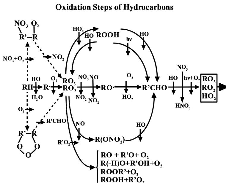
Fig. 2. Schematic presentation of the most important oxidation steps of atmospheric hydrocarbons in the polluted atmosphere. The reactions described by the dashed lines are only relevant for alkenes and alkynes.
