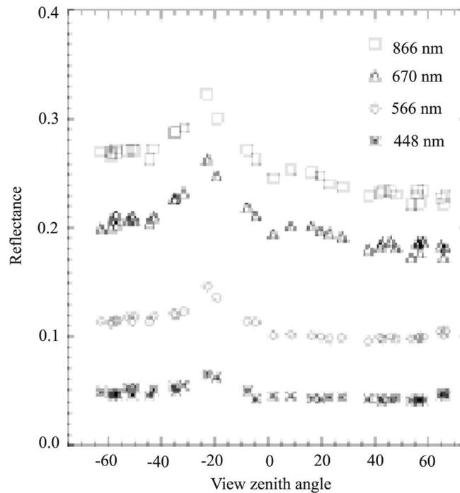
Fig. 2. Section of a BRDF in the main plane.
