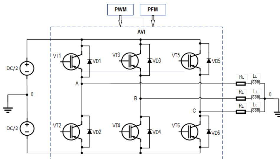
Fig. 1. Three-phase AVI circuit with PWM or PFM modulation
