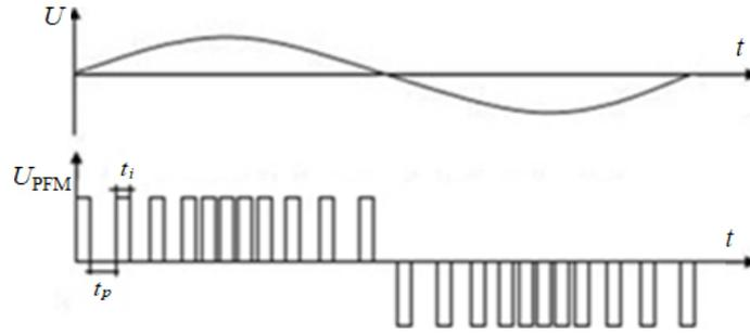
Fig. 2. Diagrams of pulse-frequency modulation formation
