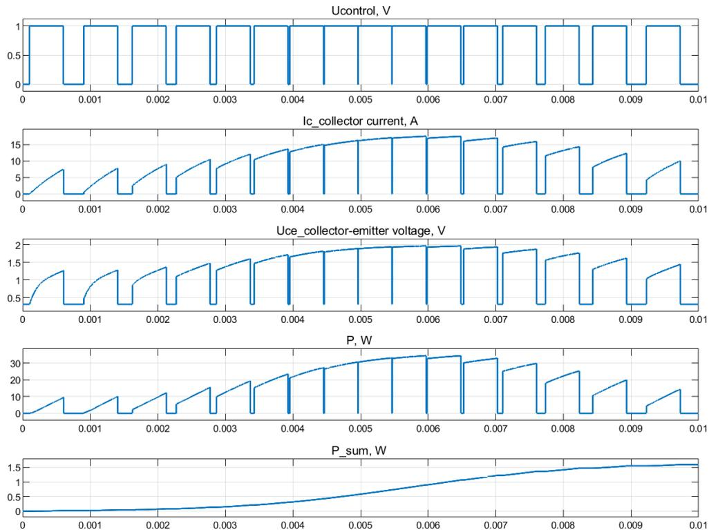
Fig. 13. Results of simulation of static losses of FS15R06XE3 module at PFM
