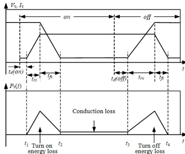
Fig. 3. IGBT transistor switching process: turn on energy loss; turn off energy loss; conduction loss (static losses in the included state);  $t_1$ – $t_2$  — power-on interval,  $t_2$ – $t_3$  — on state interval,  $t_3$ – $t_4$  — shutdown interval
