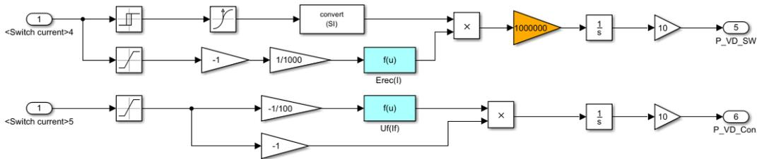
Fig. 11. Reverse diode power loss calculation unit of FS15R06XE3 type module
