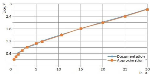
Fig. 9. Saturation voltage collector-emitter transistor type FS15R06XE3
