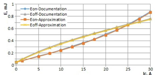
Fig. 10. Power switching characteristics of FS15R06XE3 power transistor
