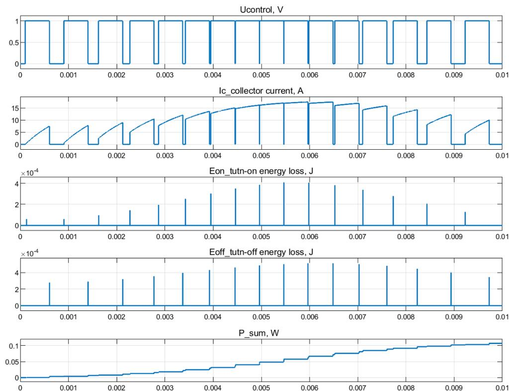
Fig. 14. Dynamic loss simulation results of FS15R06XE3 module at PFM
