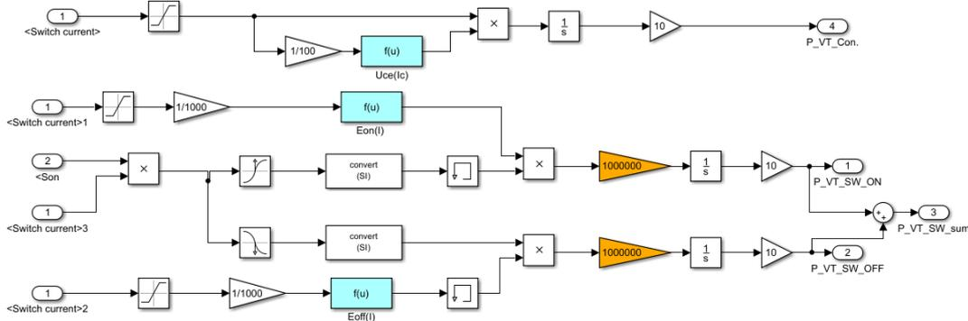
Fig. 12. Block for calculating losses IGBT/Diode module type FS15R06XE3
