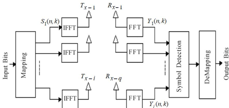
Fig. 1. Block diagram of MIMO-OFDM system
