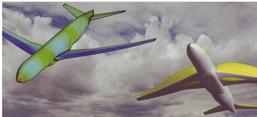
Fig. 14. The NASA Common Transonic Research Model, consisting of a wing-body-tail configuration, used in the AIAA “Drag Prediction Workshops” for comparison calculations for a Reynolds number  $Re = 2 \times 10^7$ , see, for example [27].
